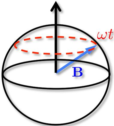
$$H(t) = \frac{\hbar\Omega}{2}\hat{\sigma}_z + \gamma(\cos\omega t\hat{\sigma}_x + \sin\omega t\hat{\sigma}_y)$$
